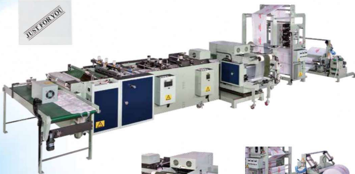
Loop handle film unit (it is adjustable with X-Left / Right, Y-Up / Down)
